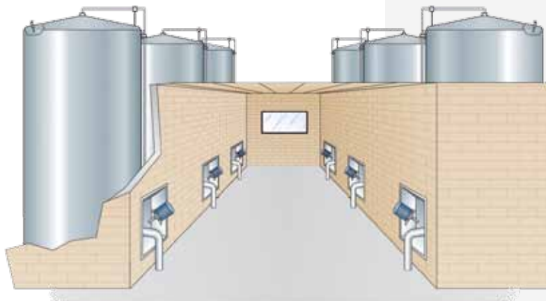
Figure 6b: Layout of outdoor silo tanks with their manholes in alcoves in the walls of a covered control station
